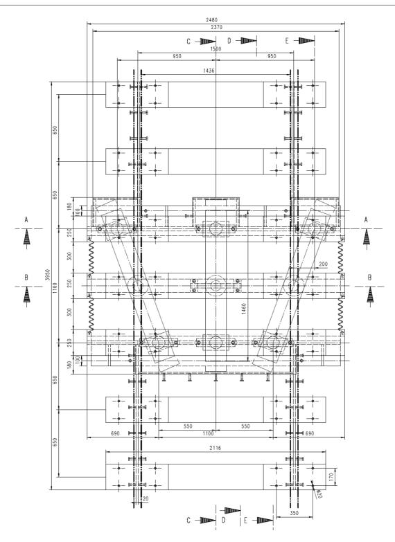
Fig: 2: Ground View of the MAURER Guided Cross-Tie System MS 1
