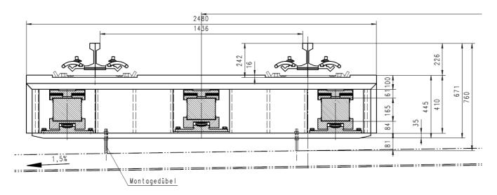
Fig: 1: Section through the MAURER Guided Cross-Tie System Type MS 1
